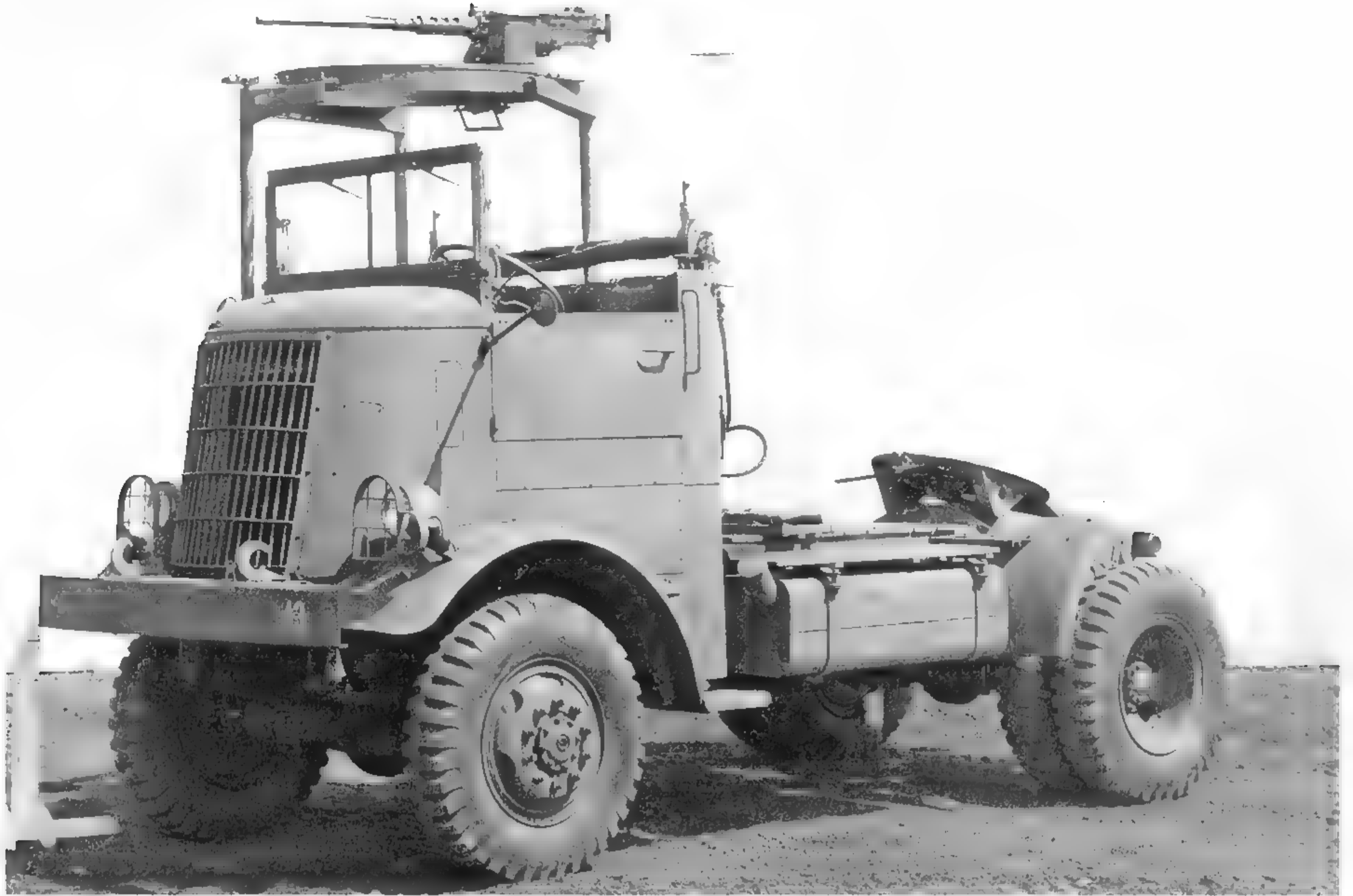
The open-cabbed trucks could also be armed. This example has been given an M57 truck mount. Regardless of mount, the weapons were designed to be operated by the assistant driver, and were only marginally effective when the vehicle was moving. (U.S. Army photo)
